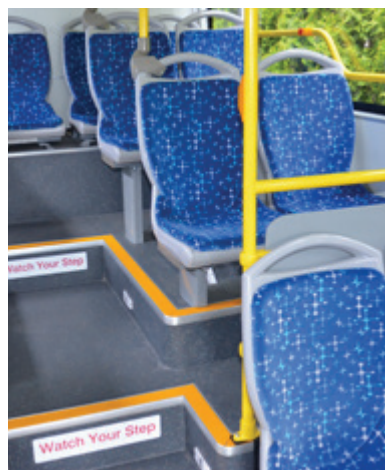
Stadium Seating Gives Feeling of Space
